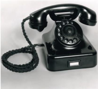
**Fig. 8.** The classic W36/38 telephone was manufactured entirely out of Bakelite, on the right a gilded special model for the Greek royal family (photos: Siemens Corporate Archives)
